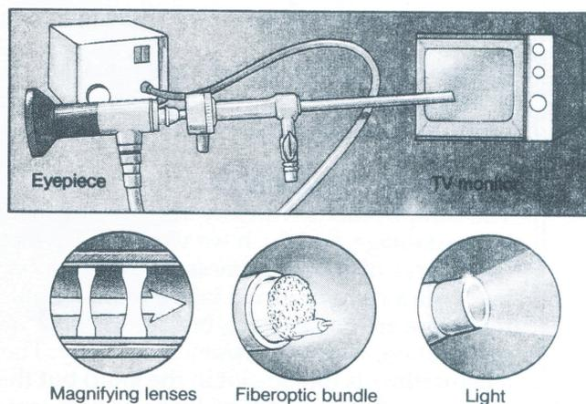
Fiber optic technology has led to the creation of the arthroscope, an instrument that allows the doctor to look directly into the knee and diagnose most problems. The arthroscope shaft (about the thickness of a knitting needle) contains coated glass fibers and a series of magnifying lenses that beam an intense, cool light into the joint and
